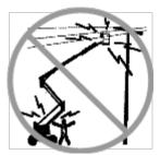
Keep away from the machine if it contacts energized power lines. Personnel on the ground or in the platform must not touch or operate the machine until energized power lines are shut off.
