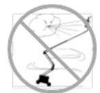
Do not raise the boom when wind speeds may exceed 28 mph/12.5 m/s. If wind speeds exceed 28 mph/12.5 m/s when the boom is raised, lower the boom and do not continue to operate the machine.
